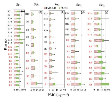
Fig. 2 In-cabin PMCs (PM<sub>2.5-10</sub> and PM<sub>2.5</sub>) in two different fractions during (a) Set<sub>1</sub>, (b) Set<sub>2</sub>, (c) Set<sub>3</sub>, (d) Set<sub>4</sub> and (e) Set<sub>5</sub>. Please note that runs taken during morning hours are marked in red colour. For the sake of clarity only positive standard deviations are shown
