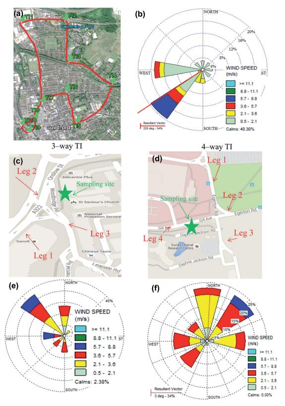
Fig. 1 (a) Map showing the location of ten TIs on the studied route for mobile measurements and the (b) wind rose diagram for the mobile monitoring period. Detailed google map showing the fixed site sampling location at (c) 3-way and (d) 4-way TIs. The wind rose diagram during the periods of fixed site monitoring at (e) 3-way and (f) 4-way TIs.
