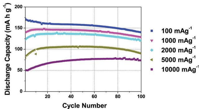
Fig. 3 Cycling performance of the 5% Mg-doped Na<sub>2/3</sub>Mn<sub>0.95</sub>Mg<sub>0.05</sub>O<sub>2</sub> cathode, evaluated at various discharge rates. The cells were cycled between 1.5 and 4.0 V vs. Na<sup>+</sup>/Na, charged at 13 mA g<sup>-1</sup> and discharged at various rates, as indicated.
