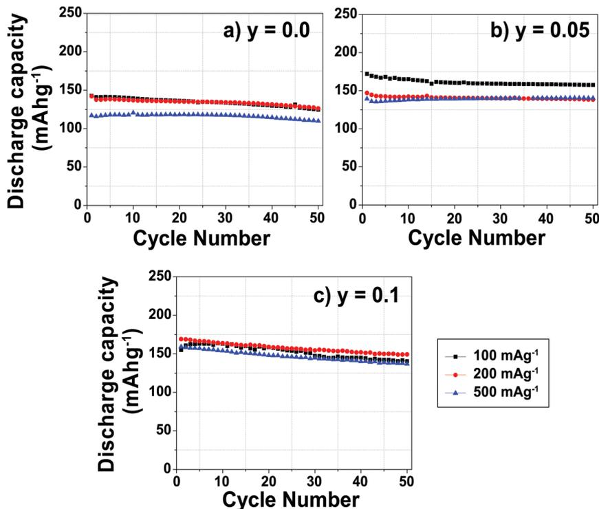
Fig. 2 Evolution of the discharge capacity as a function of the cycle number for Na<sub>2/3</sub>Mn<sub>1-y</sub>Mg<sub>y</sub>O<sub>2</sub>: (a)  $y = 0.0$ ; (b)  $y = 0.05$ ; and (c)  $y = 0.1$ . The cells were cycled between 1.5 and 4.0 V vs. Na<sup>+</sup>/Na, charged at 12 mA g<sup>-1</sup> and discharged at various rates, as indicated.
