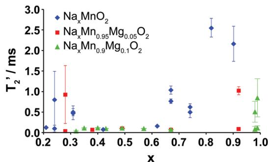
Fig. 9 Plot of the transverse NMR relaxation time ( $T_2'$ ) obtained on samples at different points along the first electrochemical charge/discharge cycle of  $\text{Na}_{2/3}\text{Mn}_{1-y}\text{Mg}_y\text{O}_2$  ( $y = 0.0, 0.05, 0.1$ ) as a function of Na content ( $x$ ). Two relaxation times are plotted on the graph when two phases or local environments were identified in the sample. Error bars for the determination of the  $T_2'$  values represent the 95% confidence intervals.
