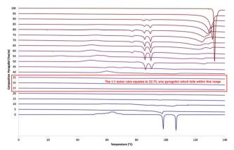
Fig. 3 Second heating phase DSC curves of ROY (0%), pyrogallol (100%) and varying compositions of ROY: pyrogallol in 5% w/w increments. The red box highlights the range of compositions in which the amorphous form is stabilised. This equates to 1:1 stoichiometry.
