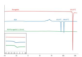
Fig. 2 Second heating phase DSC curves of pyrogallol (red), ROY (blue) and ROY: pyrogallol 1:1 grind (green). Peak onset temperatures displayed. Presence of Tg highlighted in inset.
