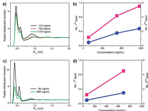
**Fig. 3** (a) Strength of cation–anion affinity in **IL-I**. (b) The numbers of counterions in 1st (blue line) and 2nd (red line) shell of **IL-I**. (c) Strength of cation–anion affinity in **IL-Cl**. (d) The numbers of counterions in 1st (blue line) and 2nd (red line) shell of **IL-Cl**. Strength of cation–anion affinity is expressed in terms of cation–anion radial distribution function, at rising concentration of **IL**.
