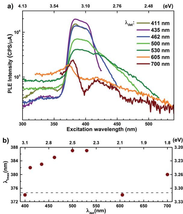
Fig. 5 (a) Semi-log plot of photoluminescence excitation spectra for different emission wavelengths for ZnO/ITO nanorods. (b) Position of maximum intensity peak ( $\lambda_{\text{max}}$ ) for different detection wavelength.
