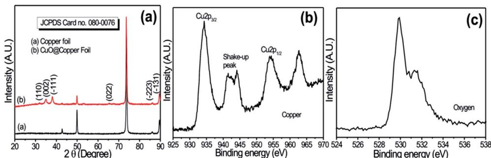
Fig. 1 (a) X-Ray diffraction patterns of copper foil and Cu foil coated with CuO electrode; (b) core-level XPS spectrum of Cu2p; (c) core-level XPS of O1s for CuO samples.
