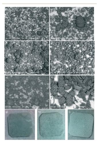
Fig. 3 SEM images of CAU-10-H synthesized directly on metallic aluminium both without using any additional acid during synthesis (a and b), using acetic acid (c and d) and using hydrochloric acid (e and f), for 100× magnification (a, c and e, scale bar indicates 100  $\mu\text{m})$  and 300× magnification (b, d and f, scale bar indicates 50  $\mu\text{m}$ ). Photographs of (2 by 2 cm) aluminium plates after synthesis without acid (g), with acetic acid (h) and with hydrochloric acid (i).
