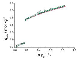
Fig. 4 Repeated H<sub>2</sub>O adsorption isotherms at 298 K of CAU-10-H supported on a metallic aluminium plate. First ( $\blacksquare$ ), second ( $\bigcirc$ ), third (▲), fourth (▼) and fifth (♠) measurements. Closed symbols depict adsorption, open desorption. Loading is presented as per total mass of sample (Al substrate + CAU-10-H).
