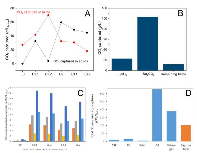
Fig. 8 (A)  $CO_2$  captured in different processing steps in brines and solids. (B) Cumulative  $CO_2$  captured for the different solids and remaining brine (B4). (C) Estimation of  $CO_2$  emissions for each electrolytic step for different possible energy sources. (D) Comparison of total  $CO_2$  emissions and  $CO_2$  capture for the overall processing strategy.
