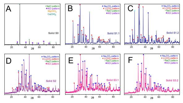
Fig. 4 X-ray diffractograms of the different solids obtained. Different diffraction peaks are assigned to reference diffraction patterns as indicated in each panel. Panels A-F show the X-ray diffractograms of solids S0, S1.1., S1.2, S2, S3.1 and S3.2, respectively.
