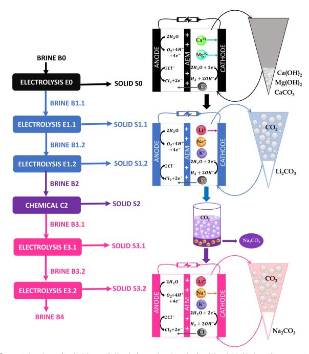
Fig. 1 Representative scheme of methodology applied in anhydrous carbon absorption from brines. In black is shown the process not-involving  $CO_2$  absorption. In blue is shown the methodology to co-obtain lithium salts. In purple is shown the chemical process for obtaining sodium crystals. In pink is shown the electrochemical process to co-obtain sodium salts.
