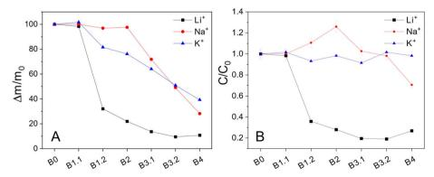
Fig. 2 (A) Percentage of initial amount of the respective cations remaining in the processed brines. (B) Concentrations (C) relative to the initial value ( $C_0$ ) of Li<sup>+</sup>, Na<sup>+</sup>, and K<sup>+</sup> in brines in different steps.
