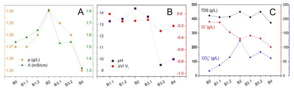
Fig. 3 Physical and chemical parameters of different brines. (A) Density (direct measurement) and conductivity (1:500 dilution). (B) pH and relative volume decrease. (C) Total dissolved solids (TDS), chloride and carbonate concentrations.
