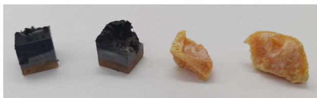
Fig. 9 Inverse vulcanised polymers showing visual evidence of the sulfur bloom effect. The polymers on the right show severe sulfur bloom all over the pieces due to being made with excessively high sulfur contents and not being cured. The polymers on the left show moderate sulfur bloom. Note how the sulfur bloom occurs toward the bottom of these polymer cubes because they were poured into a 1 cm 3 mould too early in their reaction, resulting in the denser sulfur sinking to the bottom of the cube in the absence of stirring. This led to excessively high sulfur concentrations in the bottom of the cube in comparison to the top, which could not be stabilised, resulting in sulfur bloom. Reproduced with permission from RSC Appl. Polym. , 2025, 3, 10–42. Under the Creative Commons Attribution 3.0 Unported Licence, Royal Society of Chemistry.
