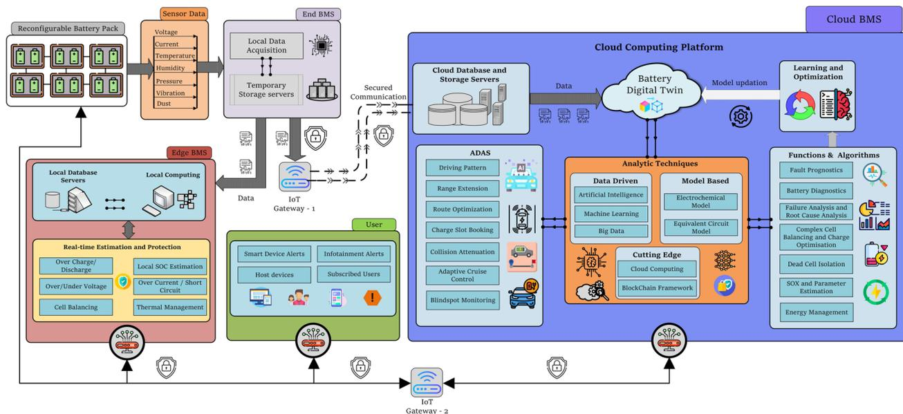
Fig. 3 Comprehensive architecture of the intelligent battery management system (IBMS) illustrating real-time multilayer (end-edge-cloud) communication. The three-layered structure (end-edge-cloud) employs hierarchical sensing and processing, with an adaptive digital twin-based cloud platform featuring an advanced analytic toolbox and blockchain technology. This setup ensures accurate prediction, prognostics, and cybersecurity for large-scale battery systems (Few icons from ref. 41).
