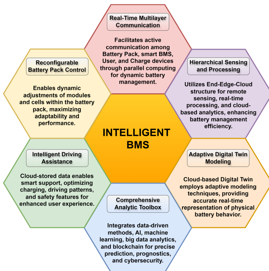
Fig. 5 Key features of the proposed intelligent battery management system (IBMS).
