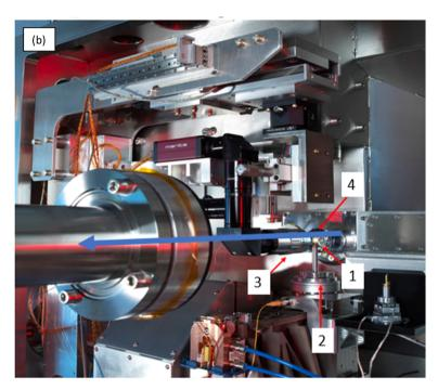
Fig. 1 (a) A schematic of the I14 hard X-ray nanoprobe beamline layout showing the major components. (b) Inside the I14 hard X-ray nanoprobe experimental hutch showing the endstation, the blue arrow indicates the X-ray beam direction. 1–4 show the position of the (1) sample mounting position, (2) scanning and rotation stages, (3) sample alignment microscope, and (4) four-element silicon drift detector (XRF detector).
