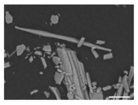
Fig. 7 SEM image of calcite prisms from *M. edulis* after dissolution of interprismatic organic matrix. Scale bar 10 um.
