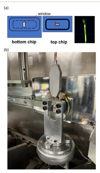
Fig. 4 (a) Sketch of MEMS liquid nanochip assembly showing the (left) bottom and top chip silicon nitride windows (perpendicular to each other), when assembled and mounted on the beamline the window area can be observed in the sample microscope (right). The windows are  $50 \, \mu m$  in width. (b) Assembled chip mounted in a liquid cell on 114 endstation.
