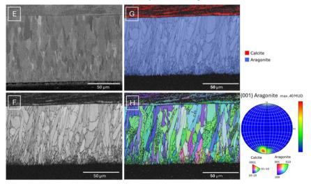
Fig. 6 (A) BSE image, (B) EBSD band contrast map, (C) EBSD phase map (D) IPF colored map and pole figure obtained on the myostracum region for the non-contaminated case. (E) BSE image, (F) EBSD band contrast map, (G) EBSD phase map (H) IPF colored map and pole figure obtained on the myostracum region for the shell from the contaminated site.
