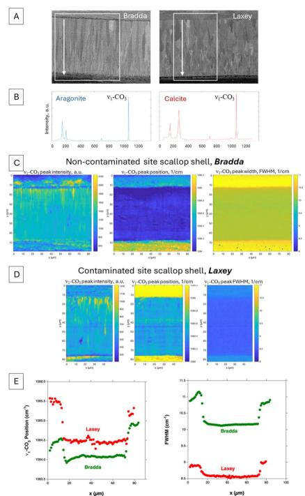
Fig. 8 (A) BSE images of a sample from non-contaminated (Bradda) and contaminated (Laxey) sites; (B) Raman spectra taken from the myostracum and foliated regions of the Bradda sample, (C)  $\nu_1$ -CO $_3$  Raman maps evaluating peak intensity, position and full width at half maximum of the Bradda and (D) and Laxey samples, (E) comparison of line profiles from top to bottom of the  $\nu_1$ -CO $_3$  Raman position and full width at half maximum for Bradda and Laxey samples.
