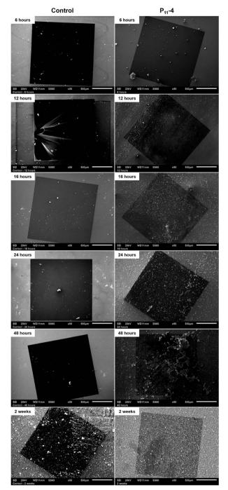
Fig. 8 Scanning electron microscopy (SEM) images of the SiN windows that were imaged on the I14 beamline to show the whole window (magnification =  $\times$ 50) at the different time points, comparing the control to the mapped SiN windows with deposited P<sub>11</sub>-4. The secondary electron detector was used at an energy of 20 kV, a working distance of 11 mm and a spot size of 60 nm.
