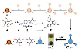
Scheme 1 Simplified linear reaction scheme for the reaction, from combination of the starting materials, A (1,3,5-triformylglucinol) and B (4-amino-L-phenylalanine). Mixing of A and B occurs in water at pH 8 and results in formation of the deprotonated non-gelating but supramolecular-fibre-assembling species  $C^{n-}$ . Acidification of  $C^{n-}$  results in protonation, giving rise to the formation of the low molecular weight gelator (LMWG) C.
