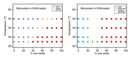
Fig. 2 Phases formed by 5% w/w monoolein in (left) EtAN— and (right) EAN—water mixtures. Schematic isothermal ternary phase diagrams drawn combining our data with available literature are shown in Fig. S11.†
