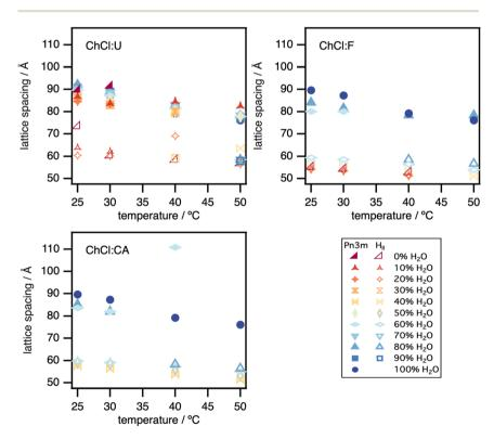
Fig. 7 Lattice spacings for the Pn3m cubic and  $H_{II}$  phases observed for monoolein in ChCl: U-water, ChCl: F-water and ChCl: CA-water mixtures. The error bars are smaller than the marker sizes. Where two  $H_{II}$  phases are observed, the larger lattice spacing is plotted.
