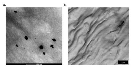
Fig. 4 Microscopy of the three-component hydrogel. (a) TEM image showing the fiber structure of the hydrogel in the background and the darker UCNP embedded within the gel. (b) SEM image providing a clearer visualization of the hydrogel structure, with the fiber arrangement being more distinct and some UCNP visible at the surface of the hydrogel.
