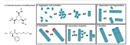
Fig. 1 (a) Chemical structure of 1,3,5-cyclohexanetricarboxamide (CTA). (b-f) Schemes summarizing processes studied in this work: (b) aggregation and nucleation, (c) dissociation and fragmentation, (d) elongation, (e) secondary nucleation, and (f) bundling.
