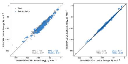
Fig. 10 Correlation of (left) force field (FIT+DMA) lattice energies and (right) force field with machine learned correction vs. DFT (B86bPBE+XDM) lattice energies. The test set (grey data points) consists of unseen crystal structures from CSP landscapes of molecules that were seen during training. The extrapolation set consists of predicted crystal structures from molecules withheld from training.
