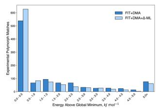
Fig. 11 Histogram of the relative energies of matches to the experimentally-determined crystal structures over all CSPs before (FIT+DMA) and after (FIT+DMA+ $\Delta$ -ML) applying the data-derived B86bPBE+XDM lattice energy correction. Separate distributions for molecules from the training and extrapolation sets are shown in the ESI.†
