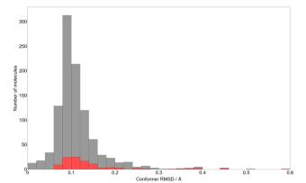
Fig. 2 A histogram of the RMSD between all atomic positions in the gas-phase optimised CSP candidate molecules, relative to their initial in-crystal conformations. The red portions of each bar indicate the molecules in that bin with spiro carbon centres.
