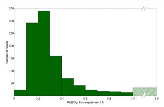
Fig. 6 A histogram of the geometric deviation between experimentally-determined crystal structures and the corresponding matching structures from CSP. The deviation is measured as the RMSD in atomic positions within 30-molecule clusters from experimental and CSP structures. Note the broken x-axis – the largest-deviation bin (green hatching) includes all matches with RMSD<sub>30</sub> greater than 1.0 Å.
