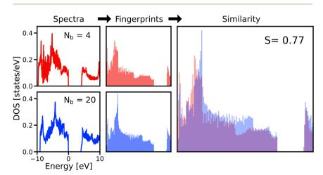
Fig. 3 Workflow for the calculation of DOS similarity. The two spectra (left panels), computed with different basis-set size  $N_{\rm b}$ , are converted to fingerprints (middle panels), for which the similarity S is calculated (right panel).
