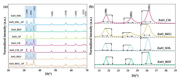
Fig. 1 XRD patterns of ZnO NPs a) before and after interaction with soil solutions, b) changes in the intensity of reflections.
