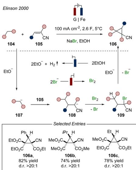
Fig. 21 Stereoselective electrocatalytic transformation of alkylidenecyanoacetates and malonate into (*E*)-3-substituted-2-cyanocyclopropane-1,1,2-tricarboxylates. Blue electrode: cathode; red electrode: anode.
