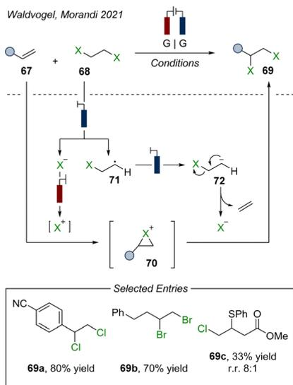
Fig. 14 Electrochemical dihalogenation of alkenes. Conditions: X = Br or X = Cl, SPh: 10 mA cm<sup>-2</sup>, 3–16 F, HFIP (1 vol%), Et<sub>4</sub>NBF<sub>4</sub> (0.2 M), r.t., CH<sub>3</sub>CN, N<sub>2</sub>. X = Cl: 4 mA cm<sup>-2</sup>, 2.5–9 F, MnCl<sub>2</sub>·4H<sub>2</sub>O (5 mol%), Et<sub>4</sub>NBF<sub>4</sub> (0.1 M), 50 °C, CH<sub>3</sub>CN, N<sub>2</sub>. Blue electrode: cathode; red electrode: anode.
