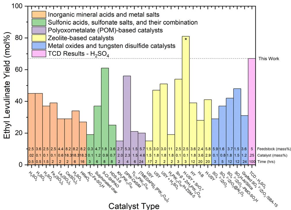
Fig. 7 Literature review of experimental yields of ethyl levulinate using various catalyst types.<sup>17,18,21,22,27,29,30,32,37–39,41–43,47,50,51,53,60,67–71</sup> All reaction systems use conventional heating and a one-pot process, excluding the H-USY-SnO<sub>2</sub> marked with a "\*" symbol, which integrates heating and spinning. The feedstock loading (mass%), catalyst loading (mass%), and reaction times are displayed at the bottom of each column.
