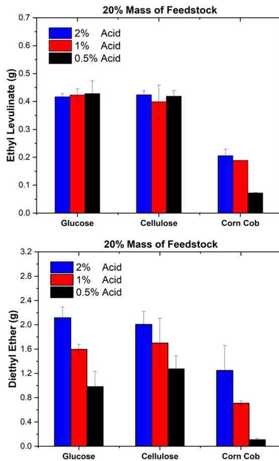
**Fig. 6** Ethyl levulinate (g) and diethyl ether (g) produced from the sulphuric acid-catalysed ethanolysis of glucose, cellulose, and corn cob (5, 10, and 20 mass %) for three different feedstock-to-acid ratios (10:1, 20:1, and 40:1) for a reaction time of 6000 minutes at 150 °C.
