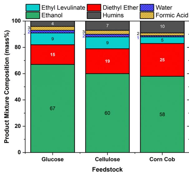
**Fig. 10** Composition of the reaction mixture (mass%) at reaction conditions that give the highest ethyl levulinate to diethyl ether ratio normalised to 100% based on the 6 main components of the reaction mixtures. The ethyl levulinate, diethyl ether, ethanol, and humins concentrations are experimentally measured. The water and formic acid concentrations are calculated stoichiometrically.
