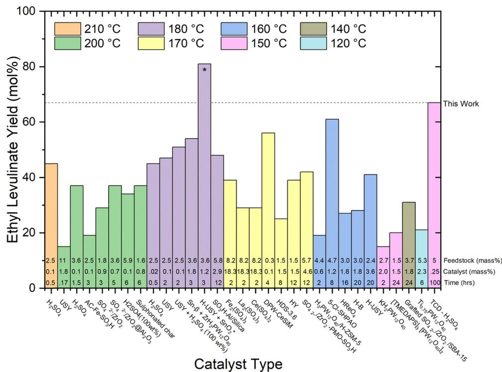
Fig. 8 Literature review of experimental yields of ethyl levulinate using various catalyst types.<sup>17,18,21,22,27,29,30,32,37–39,41–43,47,50,51,53,60,67–71</sup> All reaction systems use conventional heating and a one-pot process, excluding the H-USY-SnO<sub>2</sub> marked with a "\*" symbol, which integrates heating and spinning. The feedstock loading (mass%), catalyst loading (mass%), and reaction times are displayed at the bottom of each column.
