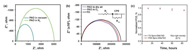
Fig. 6 (a) Nyquist plot for the devices with PAO Spiro-OMeTAD in vacuum and N<sub>2</sub>, and (b) Nyquist plot for the devices with TO and PAO Spiro-OMeTAD in O2 and dry air. (c) Light soaking stability test for the TO and PAO Spiro-OMeTAD based perovskite solar cells with a carbon electrode.
