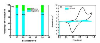
(A) Capacitive and diffusion control percentage with different scan rates of the cFl//AC electrode. (B) Proportion of surface control at 10 mV s<sup>-1</sup>.
