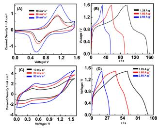
Fig. 5 Electrochemical performances of flavin-based ASCs with a KOH-PEO gel electrolyte: (A) CV plots at different scan rates from 10 to 50 mV s $^{-1}$  for **cFI//AC** ASC, (B) GCD curves at different current densities from 1.25 to 2.5 A g $^{-1}$  for **cFI//AC** ASC, (C) CV plots at different scan rates from 10 to 50 mV s $^{-1}$  for **FI//AC** ASC and (D) GCD curves at different current densities from 1.25 to 2.5 A g $^{-1}$  for **FI//AC** ASC.
