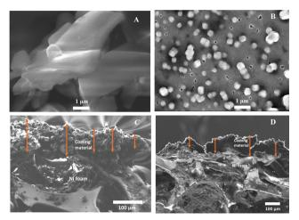
Fig. 1 FE-SEM images of (A) cFl and (B) Fl at 1 µm magnification (concentration of flavins = 0.05 mM). Cross-sectional FE-SEM images of the cFl-based electrode material (C) and Fl-based electrode material (D) at 100 µm magnification.
