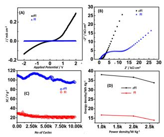
Fig. 6 (A) Linear sweep voltammetry (LSV) curves of cFl//AC and Fl//AC ASCs at a scan rate of 10 mV s<sup>-1</sup> (B) Nyquist plots for cFl//AC and Fl//AC ASCs, (C) electrochemical cycling performance of cFl//AC and Fl//AC ASCs over 10 000 cycles at a current density of 4 A g  $^{-1}$  and (D) Ragone plots for cFl//AC and Fl//AC ASCs
