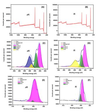
Fig. 2 (A) and (B) XPS core spectra of cFl and Fl. The deconvoluted C 1s (C) and (D) and N 1s (E) and (F) core level spectra of cFl and Fl.
