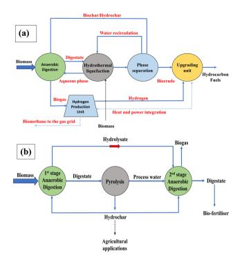
Fig. 5 (a) Flow diagram for the hybrid hydrothermal liquefaction and AD process; (b) flow diagram for the hybrid AD and hydrothermal carbonization process.
