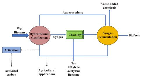
Fig. 6 Flow chart illustrating the process of hybrid gasification and syngas fermentation.
