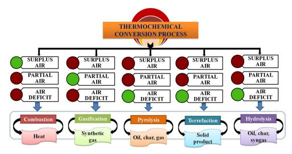
Fig. 3 Concept of thermochemical conversion processes of biomass.
