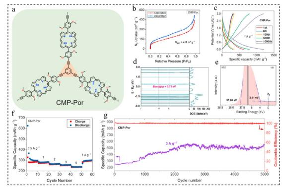
Fig. 12 (a) Structure of CMP-Por. (b) BET test for CMP-Por. (c) GCD profiles at 1 A  $g^{-1}$ . (d) Density of states of CMP-Por. (e) Ultraviolet photoelectron spectroscopy of CMP-Por. (f) Rate capability. (g) Long-term cycle life at 3 A  $g^{-1.103}$  Copyright 2022, Elsevier.
