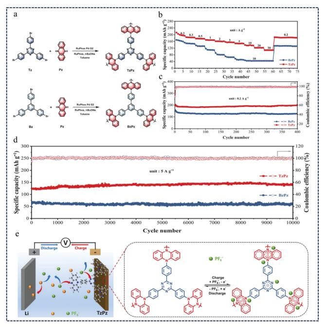
Fig. 16 (a) The synthetic reaction route of TzPz and BzPz. (b) The rate performance at current densities from 0.2 to 30 A  $g^{-1}$ . (c) Cycling performance at current densities of 0.2 A  $g^{-1}$  and (d) 5 A  $g^{-1}$ . (e) Schematic diagram of the electrochemical reaction mechanism of the TzPz-based cathode.<sup>112</sup> Copyright 2021, Wiley.
