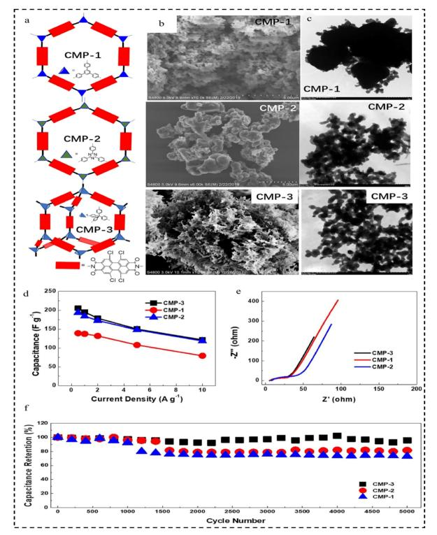
**Fig. 19** (a) Graphic representation of CMP-1, CMP-2 and CMP-3. (b) SEM images of CMP-1, CMP-2 and CMP-3. (c) TEM images of CMP-1, CMP-2 and CMP-3. (d) Specific capacitance *versus* current density curve of CMP-1, CMP-2 and CMP-3. (e) Nyquist plot of CMP-1, CMP-2 and CMP-3. (f) Cycling stability of CMP-1, CMP-2 and CMP-3 at a current density of 10 A  $g^{-1}$ .<sup>125</sup> Copyright 2022, Springer.
