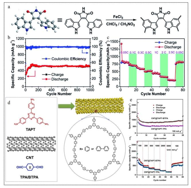
**Fig. 6** Oxidative coupling polymerization routes. (a) Synthesis of PBIM. (b) Cycle performance of CMP-PBIM. (c) The rate performance at different current densities from 0.05C to 2.5C.<sup>67</sup> Copyright 2018, Royal Society of Chemistry. Schiff-base reaction routes. (d) Synthetic route of CNT@TAPT-TPA/BTPA. (e) Cycling performance of CNT@TAPT-TPA and CNT@TAPT-BTPA. (f) Rate performance of CNT@TAPT-TPA and CNT@TAPT-BTPA. (f) Rate performance of CNT@TAPT-TPA and CNT@TAPT-BTPA.
