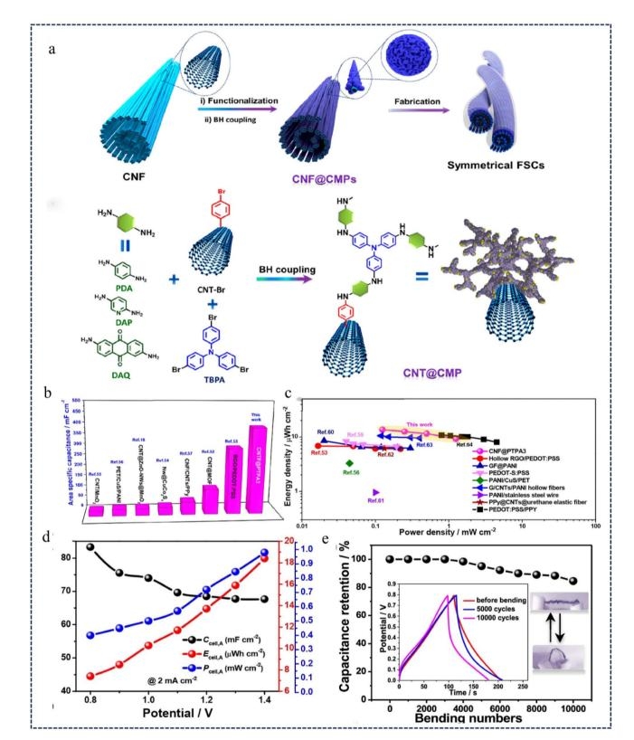
**Fig. 21** (a) Schematic illustration of the fabrication process for symmetrical fiber-shaped supercapacitors (FSCs). (b) Areal Ragone plots of the CNF@PTPA-based FSCs. (c) Comparison of electrochemical performance of CNF@PTPA FSCs with other FSCs in terms of specific capacitance. (d) GCD curves of CNF@CMP fibers. (e) Relationship between capacitance retention and bending times.<sup>131</sup> Copyright 2020, American Chemical Society.
