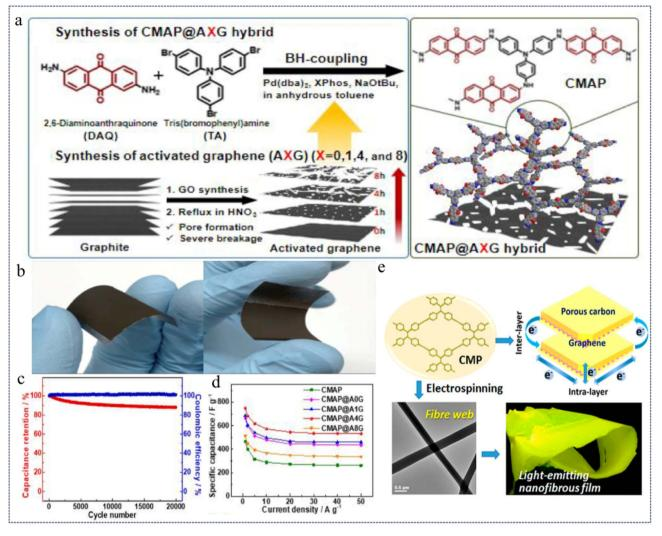
**Fig. 24** (a) Synthesis of the CMAP@XG hybrid. (b) Photographs of flexible CMAP@A4G electrodes. (c) Specific capacitance obtained at different scan rates from 1 to 50 A  $g^{-1}$ . (d) Capacitance retention and coulombic efficiency test charts at a current density of 10 A  $g^{-1.47}$  Copyright 2022, Elsevier. (e) Schematic diagram of electron transfer in graphene templated CMPs.<sup>41</sup> Copyright 2015, American Chemical Society.
