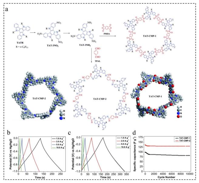
**Fig. 18** (a) The structure of TAT-CMP-1 and TAT-CMP-2. GCD curves of (b) TAT-CMP-1 and (c) TAT-CMP-2 at different current densities. (d) The relationship of the specific capacitance with cycling number for TAT-CMP-1 and TAT-CMP-2 at a current density of 10 A  $g^{-1}$  after 10 000 cycles.<sup>124</sup> Copyright 2017, Royal Society of Chemistry.
