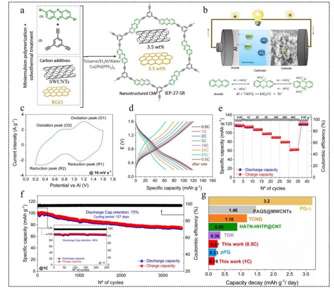
Fig. 15 (a) Synthesis strategy for IEP-27-SR mixtures. (b) Scheme of the aluminium–phenazine battery. (c) CV recorded at 10 mV s<sup>-1</sup>. (d) GCD profiles of the Al//IEP-27-SR battery. (e) Battery rate performance. (f) Long-term cycle stability of an Al//IEP-27-SR battery. (g) Capacity fade per day.<sup>107</sup> Copyright 2023, Royal Society of Chemistry.
