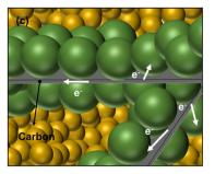
Fig. 1 Schematics of carbon–CAM composite with SEs. (a) Carbon-coated CAM mixture with SEs. (b) Mixture of CAM, CNF, and SE. (c) Carbon embedded beneath CAM and its mixture with SE.
