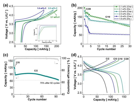
Fig. 7 Electrochemical properties of sc-NMC622/RGO composites. (a) Charge-discharge profiles of sc-NMC622/RGO composites with varied RGO contents. Inset: magnified area of the initial charging process up to 10 mA h  $\rm g^{-1}$ . (b) Cycling stability of sc-NMC622/RGO composites. (c) Cycling stability of 2.0 wt% RGO composite at C/5 and C/10. (d) Rate capability of 2.0 wt% RGO composite.
