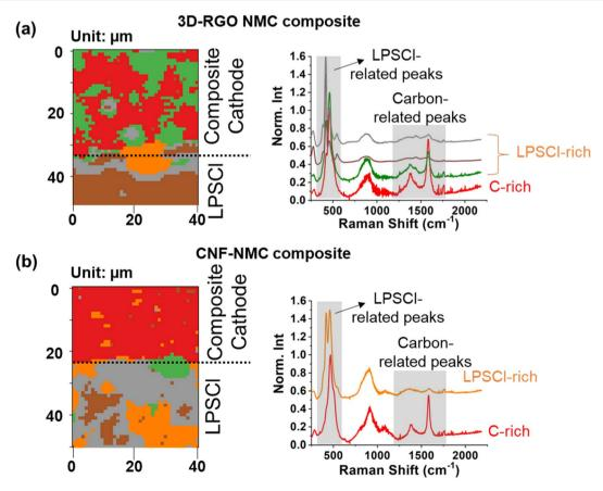
Fig. 4 Raman mapping based on K-means clustering analysis for (a) composite cathode consisting of pc-NMC811/RGO and LPSCI SE and (b) composite cathode consisting of pc-NMC811, CNF, and LPSCl SE. The black dotted line indicates the location of the composite cathode|LPSCl interface.
