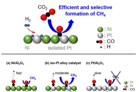
Fig. 14 Graphical representation of the adsorbed species and CO<sub>2</sub> hydrogenation over (a) Ni/Al<sub>2</sub>O<sub>3</sub>, (b) the iso-Pt catalyst, and (c) Pt/Al<sub>2</sub>O<sub>3</sub>. Adapted with permission from ref. 142. Copyright 2020 American Chemical Society.
