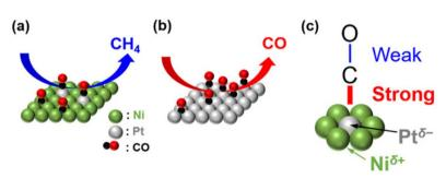
Fig. 13 Representation of the adsorbed CO species on the surfaces of the (a) iso-Pt catalyst and (b) bulk-Pt catalyst, and (c) the adsorbed CO model on a single  $Pt^{\delta-}$  atom encircled by  $Ni^{\delta+}$  atoms. Adapted with permission from ref. 141. Copyright 2019 American Chemical Society.
