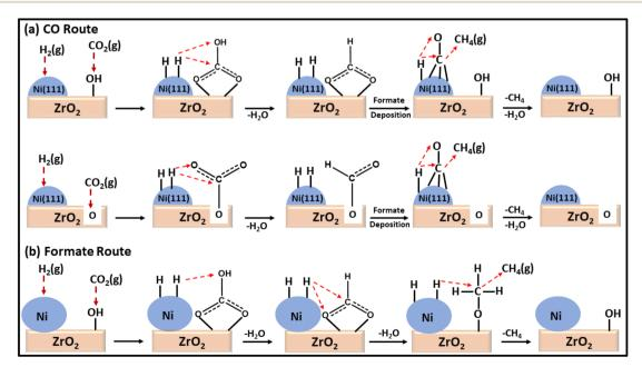
Mechanistic pathways over (a) Ni/ZrO<sub>2</sub>-plasma and (b) Ni/ZrO<sub>2</sub>-calcined catalysts for CO<sub>2</sub> methanation.
