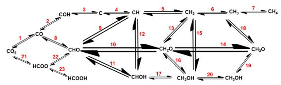
Fig. 6 Mechanistic reaction pathways for CO<sub>2</sub> hydrogenation to various reduced forms, like methane, methanol, and formic acid.
