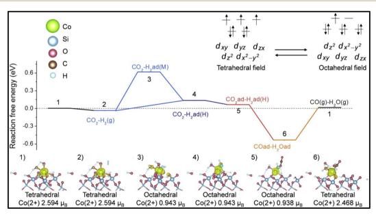
Mechanistic pathway over Co/SBA-15 catalyst for methanation. Adapted with permission from ref. 135. Copyright 2024 Elsevier B.V.
