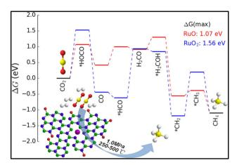
Fig. 8 Energy profile diagram for methane formation using Ru/pBN SACs. Adapted with permission from ref. 131. Copyright 2019 American Chemical Society.
