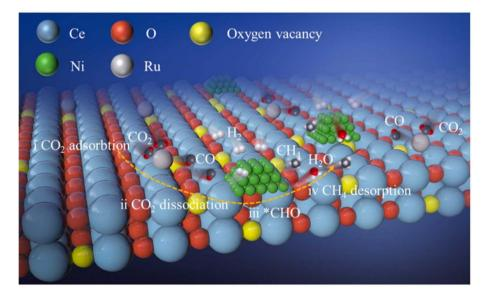
Fig. 11 Schematic representation of CO<sub>2</sub> methanation using Ru<sub>1</sub>Ni/CeO<sub>2</sub> DACs. Adapted with permission from ref. 139. Copyright 2023 Elsevier B.V.
