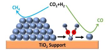
Fig. 17 CO<sub>2</sub> hydrogenation selectivity over Rh NPs and Rh/TiO<sub>2</sub> SACs.
