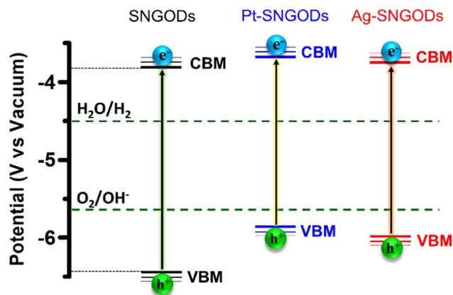
Fig. 2 Electronic-energy level diagrams of the SNGODs, Pt-SNGODs, and Ag-SNGODs in relation to the levels for  $\text{H}_2$  and  $\text{O}_2$  evolution reactions (HER and OER) in an aqueous solution of pH = 9.
