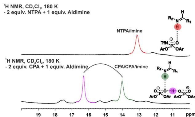
**Fig. 6** Low-temperature NMR at 180 K was used to investigate the presence of dimers in a 2 : 1 ratio of catalyst to imine. In the samples with a 2 : 1 ratio of NTPA to imine, no dimeric formation was identified. However, when employing a 2 : 1 ratio with CPA to imine, dimer formation became evident in the  $^1\text{H}$  NMR spectrum.
