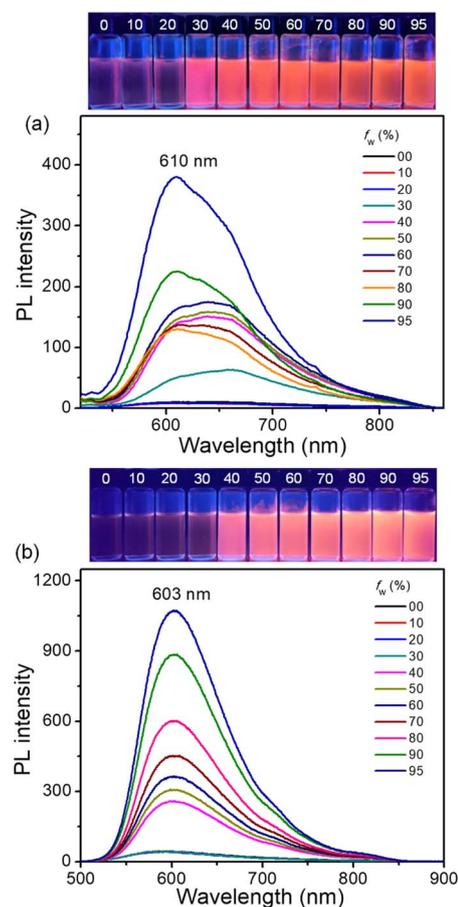
Fig. 7 Photoluminescence (PL) spectra ( $1.5 \times 10^{-5}$  M,  $\lambda_{ex} = 400$  nm) for (a) **FEM** and (b) **CATPA** in THF/H<sub>2</sub>O mixed solvents with different H<sub>2</sub>O fractions ( $f_w$ ) (insets are PL photographs of **FEM** and **CATPA** with different water fractions under 365 nm UV irradiation).
