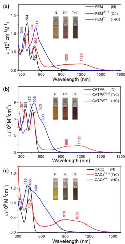
**Fig. 3** (a) UV-Vis-NIR absorption spectra for **FEM**,  $\text{FEM}^{2(+)}$  and  $\text{FEM}^{4+}$  generated by chemical titration with  $\text{AgSbF}_6$ . (b) UV-vis-NIR absorption spectra for **CATPA**,  $\text{CATPA}^{3(+)}$  and  $\text{CATPA}^{6+}$ . (c) UV-vis-NIR absorption spectra for **CACz**,  $\text{CACz}^{3(+)}$  and  $\text{CACz}^{6+}$  (insets are their photographs in DCM). N: neutral; DC: dication; TrC: trication; TeC: tetracation; HC: hexacation.
