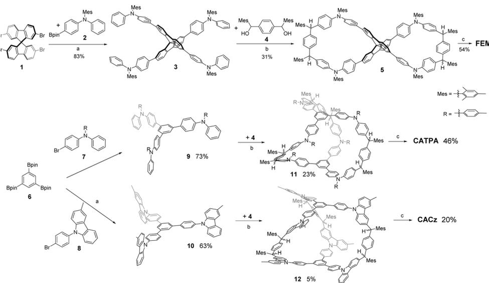
Scheme 1 Synthetic routes for **FEM**, **CATPA** and **CACz**. (a)  $\text{Pd}(\text{PPh}_3)_4$ ,  $\text{Na}_2\text{CO}_3$ , ethanol, and  $\text{H}_2\text{O}$ . (b)  $\text{BF}_3 \cdot \text{Et}_2\text{O}$  and DCM. (c) DDQ, toluene, and acetonitrile. DCM = dichloromethane; DDQ = 2,3-dichloro-5,6-dicyano-1,4-benzoquinone; and Mes: mesityl.
