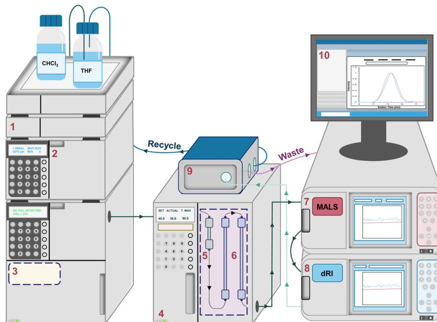
**Fig. 2** Schematic representation of a typical SEC-MALS system equipped with a (1) degassing unit, (2) solvent pump, (3) autosampler, (4) column oven, (5) guard column, (6) separation columns, (7) MALS detector, (8) dRI detector, (9) solvent recycling system, and (10) computer interface.
