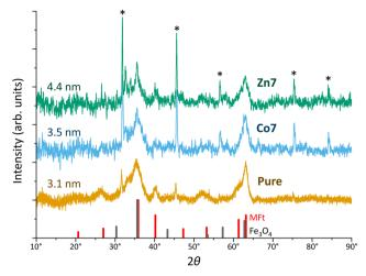
Fig. 4 X-ray diffraction patterns of magnetoferritin (pure) and doped (Co7 and Zn7) samples using Cu-K $_{\alpha}$  radiation. Runs I-III were pooled. Sharp peaks indicated by asterisks originate from residual NaCl after drying. Crystallite sizes obtained from the Scherrer analysis are given on the left. Sticks in black and red indicate the angles and intensities for Fe $_3$ O $_4$  and MFt powder samples, respectively. Diffractograms are shifted vertically for better visibility.
