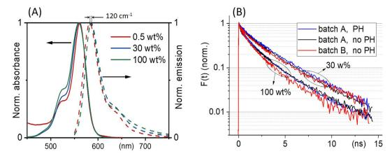
Fig. 3 (A) ONPs steady-state absorption and emission spectra as a function of R18/F5-TPB loading. (B) Comparison of the fluorescence decay kinetics recorded with (PH) or without (no PH) pinhole, at low excitation power where no EEA occurs, for two batches A and B of nanoparticles ONP30 and ONP100. The results of the tri-exponential fits of all these curves are disclosed in Table 1.
