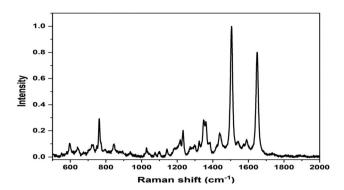
Fig. 2 SERS spectrum of L3@SERS-NS where the dominant features are those of the SERS spectrum of TR-SH at 1505 and 1649  $\rm cm^{-1}$ .
