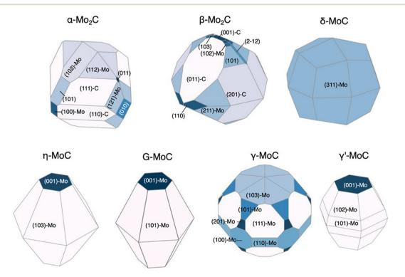
Fig. 6 DFT-computed Wulff constructions of the equilibrium particle morphologies of different molybdenum carbide phases at  $\Delta\mu_{\rm C} = -0.15$  eV using NN-identified facets. This figure has been reprinted from ref. 93 with permission from the American Chemical Society, copyright 2021.
