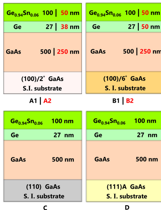
Fig. 1 Cross-sectional schematics of \text{Ge}_{0.94}\text{Sn}_{0.06}/\text{Ge}/\text{GaAs} heterostructures with differently orientated and misoriented semi-insulating (S. I.) GaAs substrates, analyzed in this work: A1 (A2) – 100 (50) nm thick epitaxial \text{Ge}_{0.94}\text{Sn}_{0.06} layer grown on 27 (38) nm Ge buffer with (100)/2° orientation; B1 (B2) – 100 (50) nm thick epitaxial \text{Ge}_{0.94}\text{Sn}_{0.06} layer grown on 27 (50) nm Ge buffer with (100)/6° orientation; C and D – 100 nm thick \text{Ge}_{0.94}\text{Sn}_{0.06} grown on 27 nm Ge buffer with (110) and (111)A orientations, respectively. The \text{Ge}_{0.94}\text{Sn}_{0.06} epilayers are ~0.81% compressively strained.
