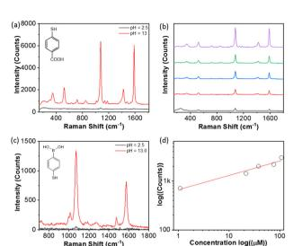
Fig. 5 (a) SERS response of PAH-grafted AuNPs for 4-MCTA at pH values of 1 and 13. (b) SERS response of 4-MCTA at a concentration range of 1-100 µM with PAH-grafted AuNPs. (c) SERS response of 4-MCBA at pH values of 1 and 13 with PAH-grafted AuNPs. (d) Plotting the peak intensity at 1074 cm<sup>-1</sup> at a pH value of 13 against the concentration of 4-MCBA.
