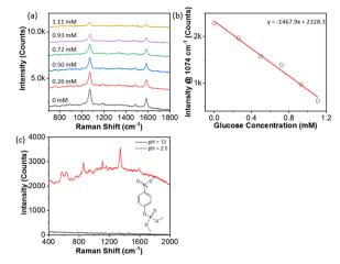
**Fig. 8** (a) Glucose detection using 4-MCBA with PAA-grafted AgNPs at concentrations of 0 mM to 1.11 mM of glucose in addition to 0.5 M  $\rm H_3PO_4$  solution. (b) Plotting the peak intensity of 4-MCBA at 1074 cm<sup>-1</sup> vs. glucose concentrations of 0 mM to 1.11 mM. (c) Detection of methyl parathion using PAA-grafted AgNPs at a concentration of 17 ppm after adding  $\rm H_3PO_4$ .
