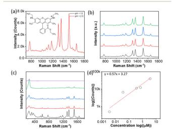
Fig. 6 (a) SERS response of PAA-grafted AgNPs for R6G at 0.36  $\mu$ M. (b) SERS spectra of R6G PAA-grafted AgNPs at pH 2.5 for different solution spots. (c) SERS response of R6G in the concentration range of 3.6 nM-3.6 µM with PAA-grafted AgNPs. (d) Plotting the peak intensity at 1341 cm<sup>-1</sup> against the concentration of R6G.
