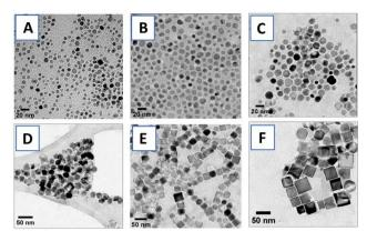
Fig. 2 Representative transmission electron microscopy (TEM) images of IONPs synthesized using thermal decomposition of Fe(acac)<sub>3</sub>: (A) 7.3  $\pm$  1.4 nm, (B) 11.0  $\pm$  2.0 nm, (C) 15.4  $\pm$  2.1 nm, (D) 19.1  $\pm$  2.3 nm nano-octahedrals, (E) 27.4  $\pm$  3.6 nm and (F) 33.4  $\pm$  4.9 nm nanocubes ( $\pm$  denotes standard deviation,  $n \ge 100$ ).
