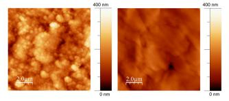
Fig. 2 Non-contact representative AFM images (10  $\mu m \times$  10  $\mu m$ ) of GL-coated PCL scaffolds (left) and the PCL substrate (right).
