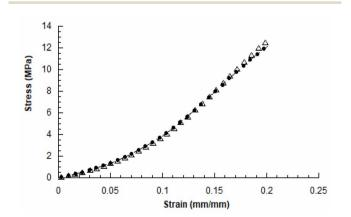
Fig. 3 Typical stress-strain curves obtained for 3D AM PCL ( $\bullet$ ) and GL-coated PCL ( $\triangle$ ) scaffolds (rate of 1 mm min<sup>-1</sup> and final strain of 20%).
