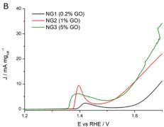
Fig. 8 (A) HER LSVs and (B) OER LSVs registered in KOH 0.1 M at 1 mV s<sup>-1</sup> and 1600 rpm for NG1 (black curve), NG2 (red curve) and NG3 (green curve) samples.
