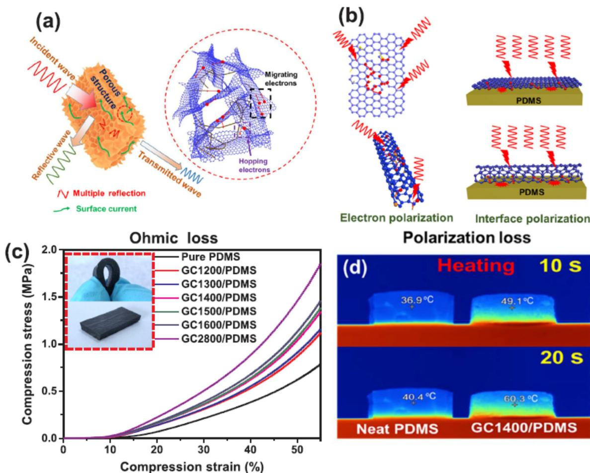
**Fig. 8** (a and b) Schematic diagram of the EM shielding mechanism of the GC/PDMS composites. (c) Compression stress–strain curves of GC1400/PDMS and neat PDMS. The inset shows the optical images of GC1400/PDMS and the bent GC1400/PDMS. (d) Infrared thermography images of GC1400/PDMS and neat PDMS in heating for 10 s and 20 s (the hot stage with a temperature of 150 °C); reproduced with permission from ref. 90, copyright reserved Elsevier 2020.
