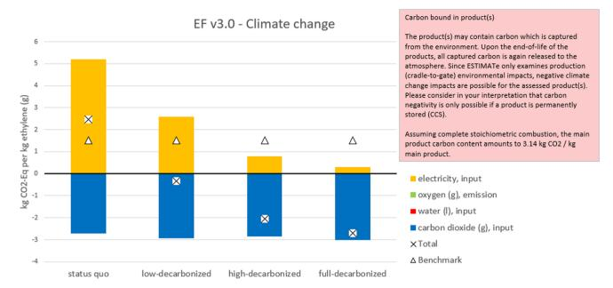
Fig. 3 Climate Change Impact of the Best-Case Assessment of electrochemical CO<sub>2</sub> reduction to ethylene in the ESTIMATe tool. The different bars correspond to the different background system scenarios defined in section 2.4.
