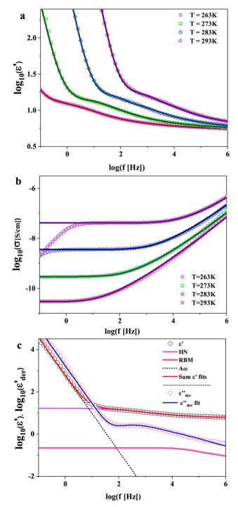
Fig. 4 (a and b) The real parts of the complex dielectric,  $(\varepsilon^*(\omega) = \varepsilon'(\omega) - i\varepsilon''(\omega))$ , and complex conductivity functions,  $(\sigma^*(\omega) = \sigma'(\omega) + i\sigma''(\omega))$ , for PVB MeTFSI polymerized ionic liquid at the selected temperatures as indicated. The lines denote fits obtained by combining the Havriliak-Negami function to account for re-orientational ion dynamics,
