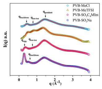
Fig. 3 The wide-angle X-ray scattering intensity *versus* the wave vector, q, for the polylLs investigated in the current work at 300 K. The arrows indicate the peak positions associated with the backbone-ion, and pendant-correlation distances. The red solid lines are fits obtained using asymmetric Lorentzian functions.
