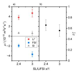
Fig. 3 (a) Mobility data of SL/LiFSI = x/1 with x = 2.4 and 3 for Li<sup>+</sup> (red dots), FSI<sup>-</sup> (blue squares) and SL (grey triangles) and (b) the resulting Li<sup>+</sup> transference numbers  $t_+^{\mu}$ .
