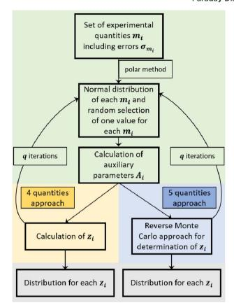
Fig. 2 Scheme of the software algorithm for the calculation of the Onsager coefficients and the thermodynamic factor. Part 1 is highlighted in green, part 2 is highlighted in yellow (4-quantities approach) and blue (5-quantities approach), and part 3 is highlighted in grey.
