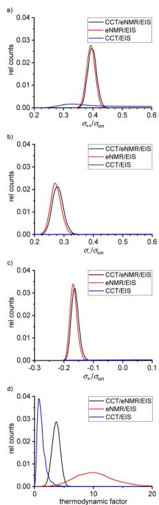
Fig. 6 Calculated distributions of the normalized Onsager coefficients (a)  $\sigma_{++}/\sigma_{\rm ion}$ , (b)  $\sigma_{--}/\sigma_{\rm ion}$ , (c)  $\sigma_{+-}/\sigma_{\rm ion}$  and (d) of the thermodynamic factor for the SL/LiFSI 3/1 electrolyte.
