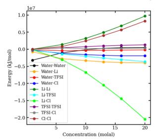
Fig. 8 Coulomb interaction energies in kJ mol<sup>-1</sup> between pairs of species in aqueous LiCl-LiTFSI biphasic systems, plotted against molal concentration.
