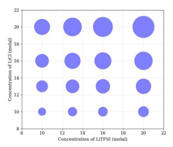
Fig. 9 Bubble plot, where the size of circles is linearly proportional to the experimental interfacial tension between liquid phases in a biphasic system, with molal concentration of LiCl on the *y*-axis, and molal concentration of LiTFSI on the *x*-axis.
