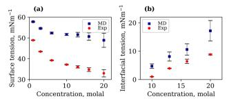
Fig. 2 Calculated (blue) and experimentally measured (red) interfacial tensions with respective errors in mN  $\rm m^{-1}$ , for (a) LiTFSI-vapour systems of 1, 3, 6, 10, 13, 16 and 20 molal, and (b) LiTFSI-LiCl systems of 10, 13, 16 and 20 molal (both phases). Errors are calculated based on block averages over 5 blocks using the full-precision averages.
