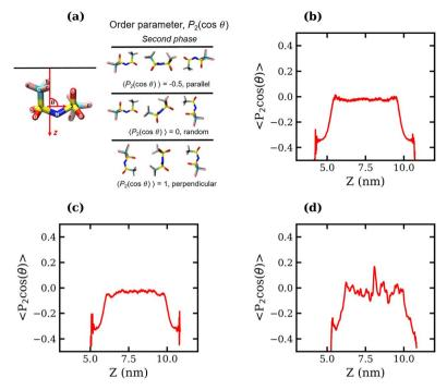
Fig. 5 Average order parameter,  $\langle P_2(\cos \theta) \rangle$ , of TFSI<sup>-</sup> anions measured as the second Legendre polynomial of  $\theta$ , the angle between the S-S vector and interface normal (a), plotted against the Z coordinate for the (b) 1 molal, (c) 10 molal and (d) 20 molal liquid vapour systems.
