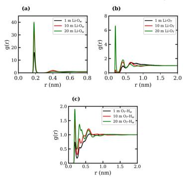
Fig. 1 Radial distribution functions of (a) Li<sup>+</sup> with O (water), (b) Li<sup>+</sup> with O (TFSI<sup>-</sup>), and (c) O (TFSI<sup>-</sup>) with H (water), all shown for the 1 molal LiCl aqueous system (black), the 10 molal system (red) and the 20 molal system (green).
