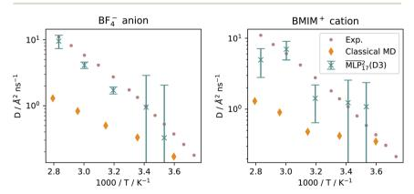
Fig. 6 Arrhenius plot of the diffusion coefficients at different temperatures. Experimental values are taken from Hayamizu *et al.*,<sup>53</sup> and results for classical MD are replicated from Bagno *et al.*<sup>66</sup>
