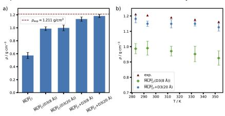
Fig. 7 Densities obtained from NPT simulations in comparison to experimental values taken from Hayamizu  $et~al.^{53}$  (a) Densities produced by models differing in the way the dispersion correction was learned or added for  $BMIM^+BF_4^-$  at 283 K. (b) Comparison of densities across temperatures for three of these models. Error bars indicate 95% confidence intervals.
