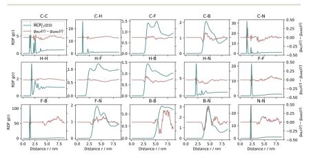
Fig. 3 Comparison of RDFs at 353 K for 16 ion pairs of BMIM $^+$ BF $_4^-$  from 20 ns MLP MD and 10 ps AIMD simulations.
