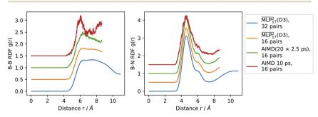
Fig. 4 RDF of B-B and B-N pairs. The B-B RDF shows significant structure, which is smoothed out over the 20 ns.
