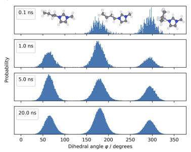
Fig. 5 Dihedral angle distribution of an *n*-butyl chain in a single BMIM<sup>+</sup> cation plotted over different simulation time scales. Molecules are visualized using the ZnDraw<sup>61</sup> package.
