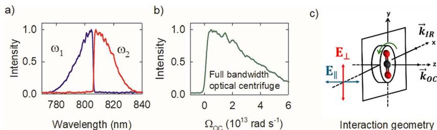
Fig. 2 (a) Spectra of oppositely-chirped optical centrifuge pulses. (b) Profile of the optical centrifuge as a function of angular frequency using the full bandwidth of  $\omega_1$ . (c) Geometry of the interaction region where optically centrifuged molecules are probed with polarization-sensitive transient IR absorption spectroscopy. The IR polarizations are labeled relative to the z-axis.
