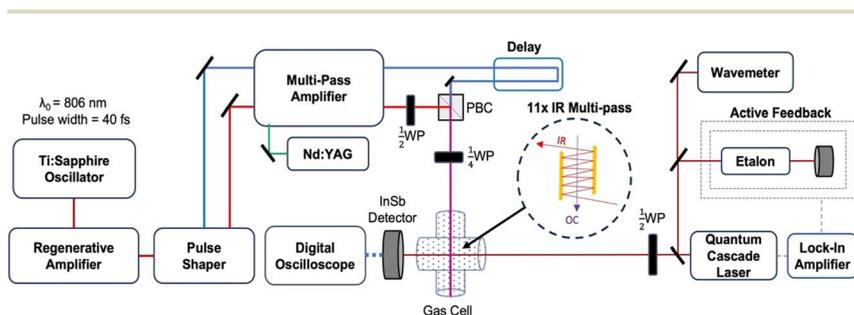
Fig. 1 Schematic diagram of the optical centrifuge and high-resolution transient IR absorption spectrometer. The pair of optical centrifuge pulses have orthogonal linear polarization after the  $\frac{1}{2}$ -wave plate ( $\frac{1}{2}$ WP) and opposite circular polarization after the  $\frac{1}{4}$ -wave plate ( $\frac{1}{4}$ WP). The IR  $\frac{1}{2}$ -wave plate is used to control the polarization of the IR probe.
