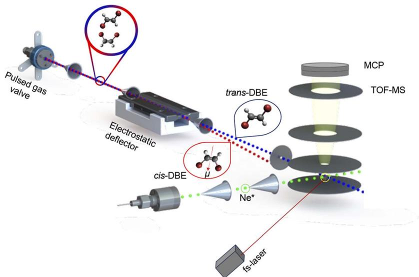
Fig. 1 Schematic of the crossed-molecular-beam experiment used in the present study. The polar *cis* and apolar *trans* stereoisomers of 1,2-dibromoethene (DBE) were separated from a mixture using an electrostatic deflector and overlapped with a second beam containing metastable neon atoms ( $\text{Ne}^*$ ) in the extraction region of a time-of-flight mass spectrometer (TOF-MS) to study isomer- and rotationally-resolved chemi-ionisation (CI) reactions. See text for details.
