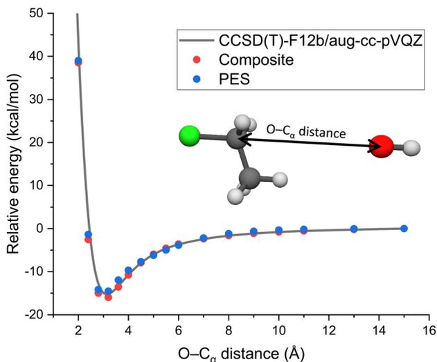
Fig. 3 Potential along the O–C<sub>α</sub> distance of OH<sup>−</sup> + CH<sub>3</sub>CH<sub>2</sub>Cl keeping the reactants at fixed equilibrium geometries obtained by the CCSD(T)-F12b/aug-cc-pVQZ and composite (eqn (3)) *ab initio* levels of theory as well as on the analytical PES.
