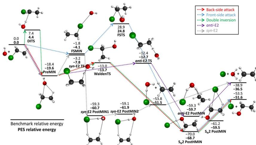
Fig. 2 The schematic energy diagram of the  $\text{OH}^- + \text{CH}_3\text{CH}_2\text{Cl}$   $\text{S}_{\text{N}}2$  and E2 reactions; the classical relative energies ( $\text{kcal mol}^{-1}$ ) obtained on the PES developed in this work are in comparison with the benchmark, CCSD(T)-F12b/aug-cc-pVQZ single-point results (ref. 20).
